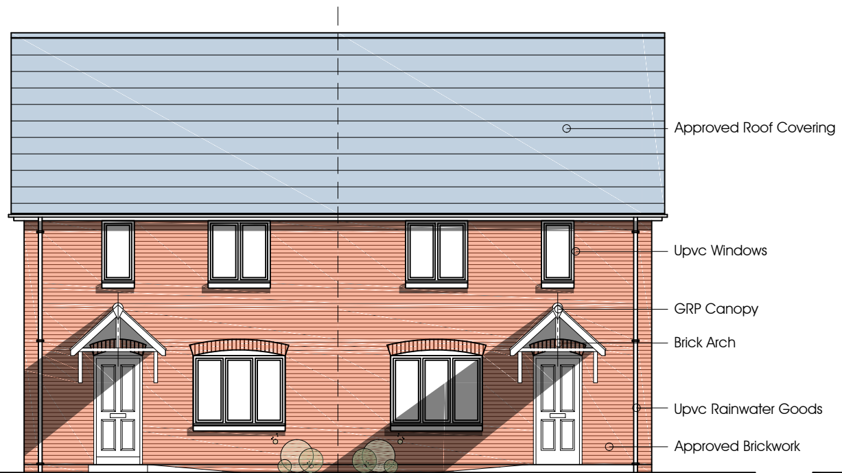
FRONT ELEVATION Typical 2 Bed House
