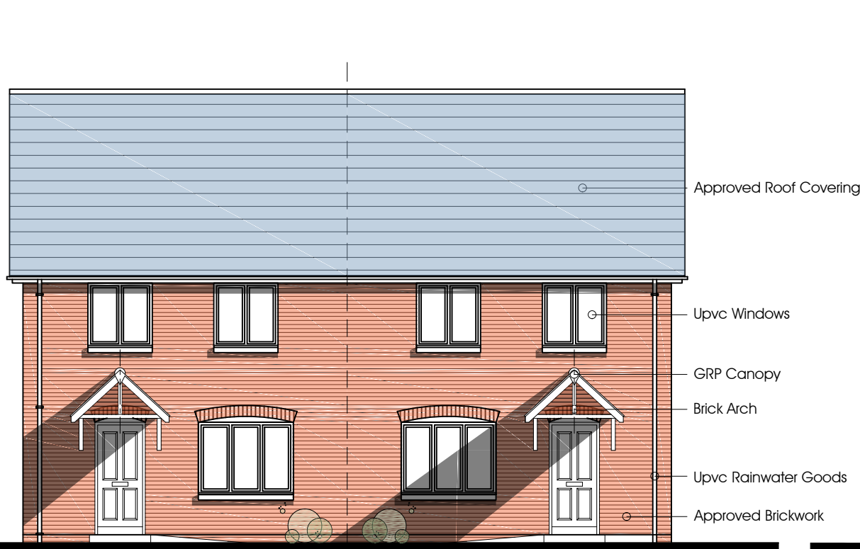
FRONT ELEVATION Typical 3 Bed House
